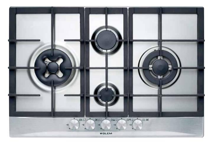
The design of the cast iron trivets to the full width of the cooktop maximizes the cooking area. On the left hand side there is a dual control wok burner which allows for a simmer rate from 1 Mj/h right up to 16 Mj/h. On the right hand side there is a 14.0 Mj/H triple ring wok burner. The burners have been spaced to allow for stir frying in a wok while cooking rice on the other burner.
