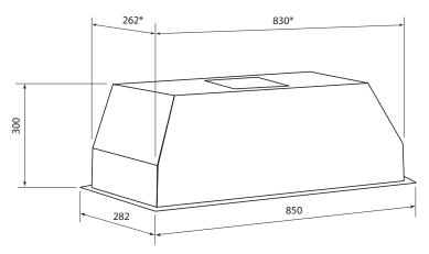
\* allow 5mm clearance for installation
