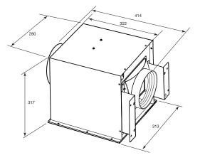
Remote fan motor goes into ceiling space. NOTE: Check that you home has a ceiling space above the kitchen to locate the motor.
